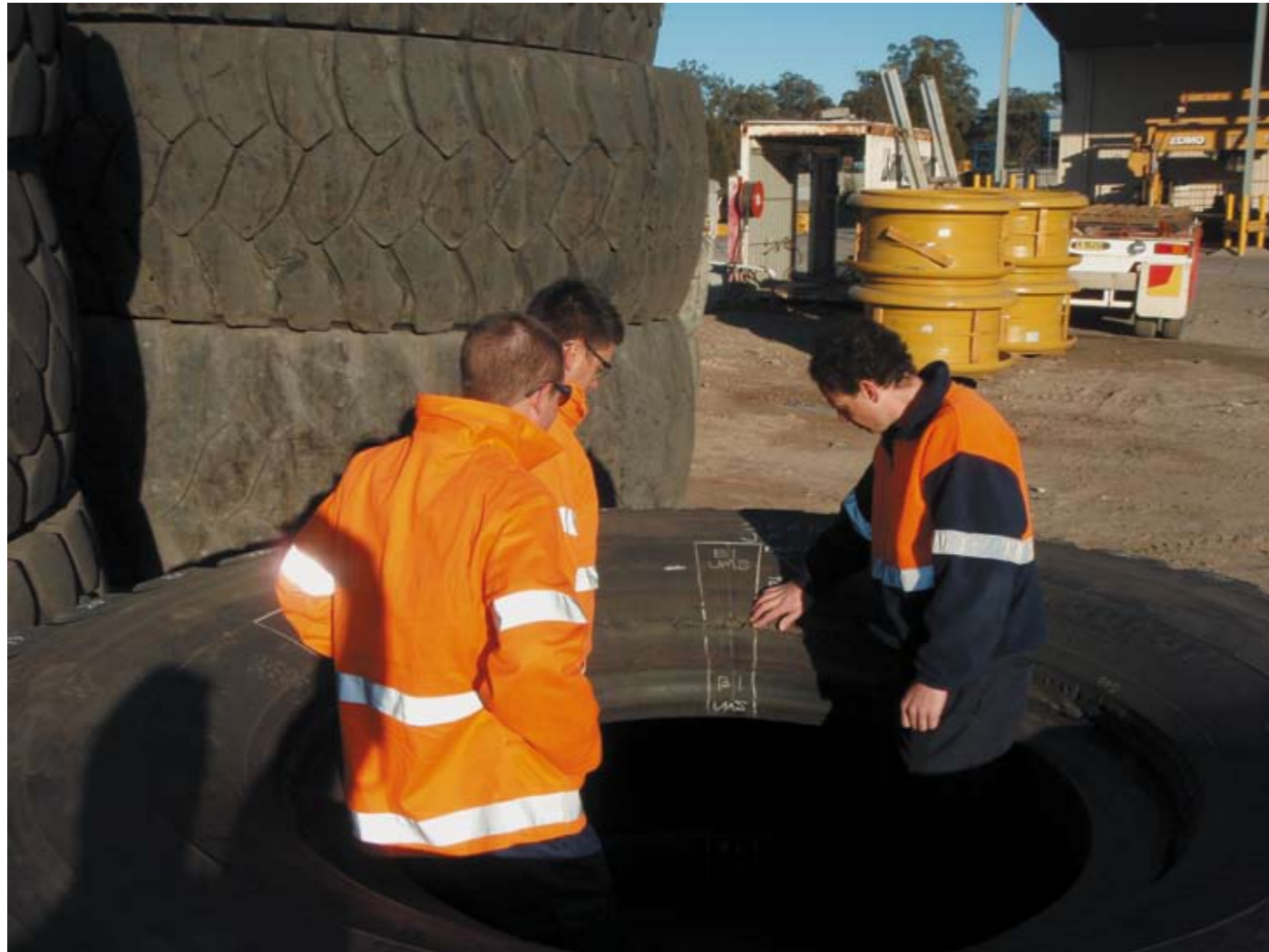
Damage to this tyre resulting from under-inflation meant it had to be discarded.
