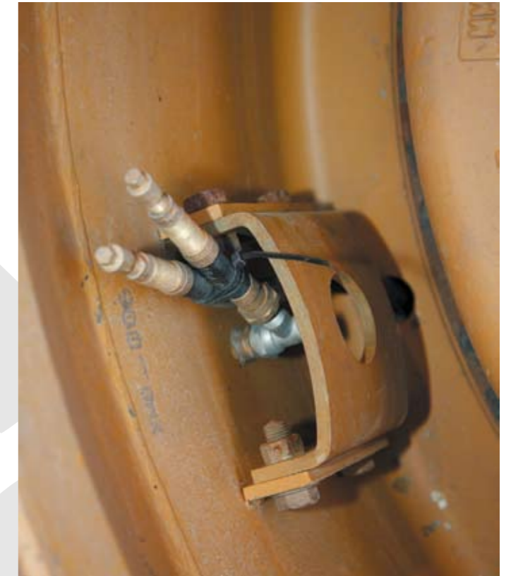
Valve caps are simple way to maintain tyre pressures. Valves without caps will leak.
