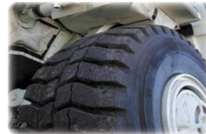
Good site management practices, including ensuring loading and haulage areas are kept smooth and clean, will assist greatly in prolonging tyre life.
