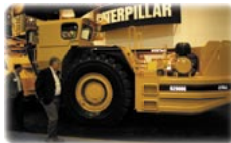
Cat Elphinstone's R2900G Xtra underground loader fitted with low-profile Bridgestone 35/65R33 tyres and Topy rims – a combination developed in Australia.
