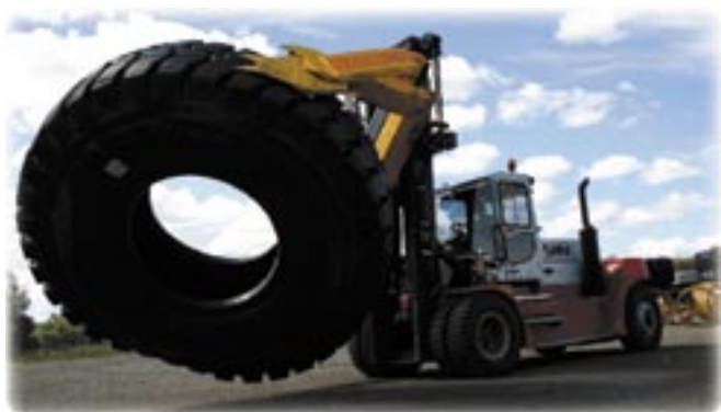
Bridgestone's recently commissioned tyre-handling forklift, on site at Bulga Coal.
