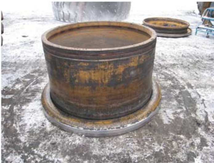
The photo on the left shows a rim treated with Seal-Zit once the tyre had been removed following several thousand hours of use; compare the surface quality with that on the right, which had not been treated at all.
