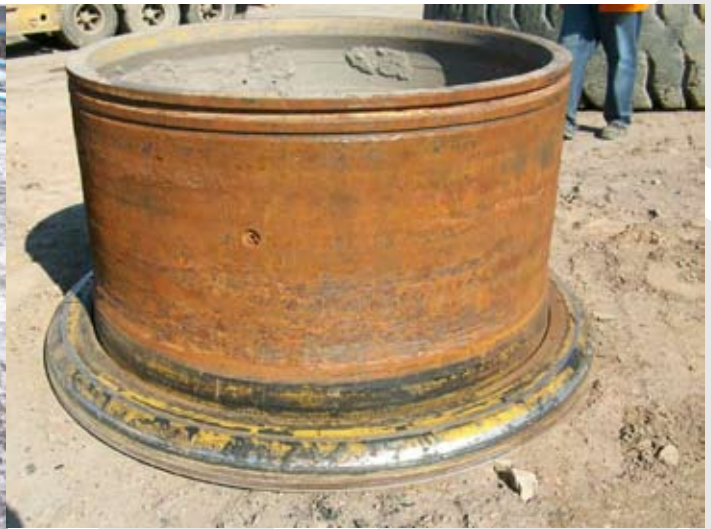
The photo on the left shows a rim treated with Seal-Zit once the tyre had been removed following several thousand hours of use; compare the surface quality with that on the right, which had not been treated at all.
