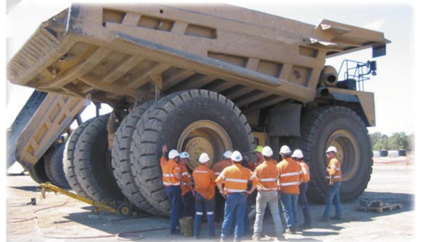
New standards recommend that mines, quarries and construction sites set their own maximum pressures for removing and working on tyres, depending on what is safe and appropriate working practice for each piece of equipment.
