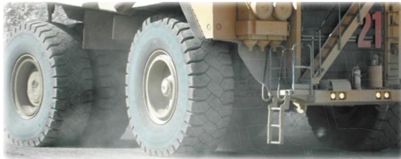
Bridgestone's E4 class VRDP series tyres are designed for operations on abrasive or harsh surfaces.
